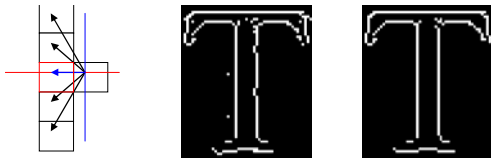
Figure 7. Adjustment of edge position. a) The adjustment. Blue line as the edge direction, red line as the normal direction and the red square is the new position post adjustment; b) Edge position before adjustment; c) Edge position after adjustment
