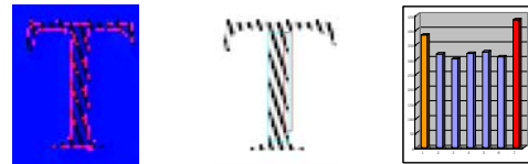
Figure 5. The edge position detection result and analysis. a) The position result detected by the Gaussian template. Red pixels are edge position result and black pixels are image data. b) The unstable area enclosed by red line. c) The statistic information of the gray value within the area enclosed by blue line in b)
