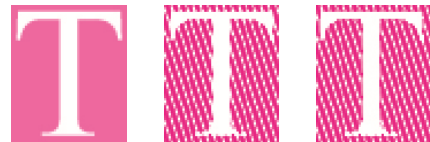
Figure 10. From left to right: the original image, halftone image, result of enhancement. The case of lighter text (font size: 10) on darker background. C: 0%; M: 75%; Y: 0%; K: 0%.
